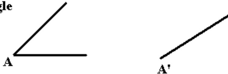
**Step 1: Draw an arbitrary arc with center A of the given angle, then with the same compass setting redraw the arc with center A'.**
